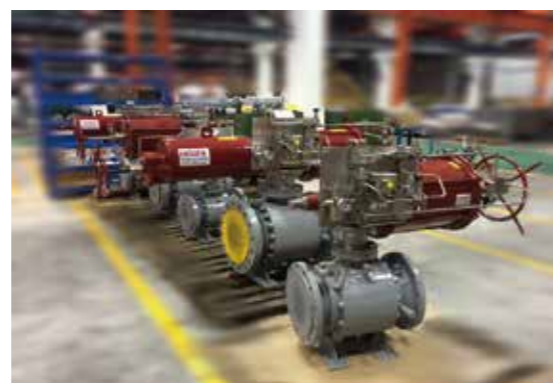
10" #150 Ball Valve with Pneumatic Spring Return Actuator for ESD service with Partial Stroking System
