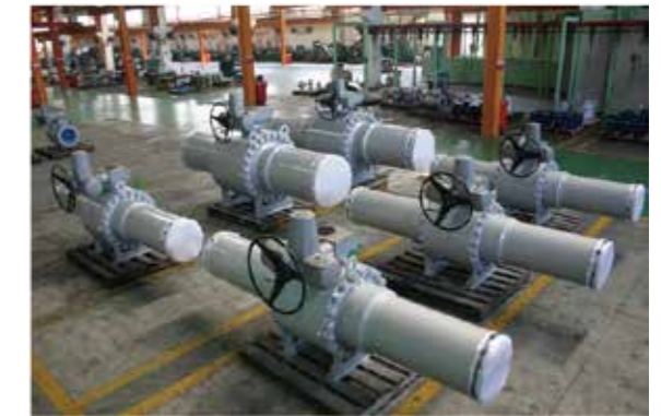
12" #150 Trunnion Mounted Ball Valve with Electric Actuator
